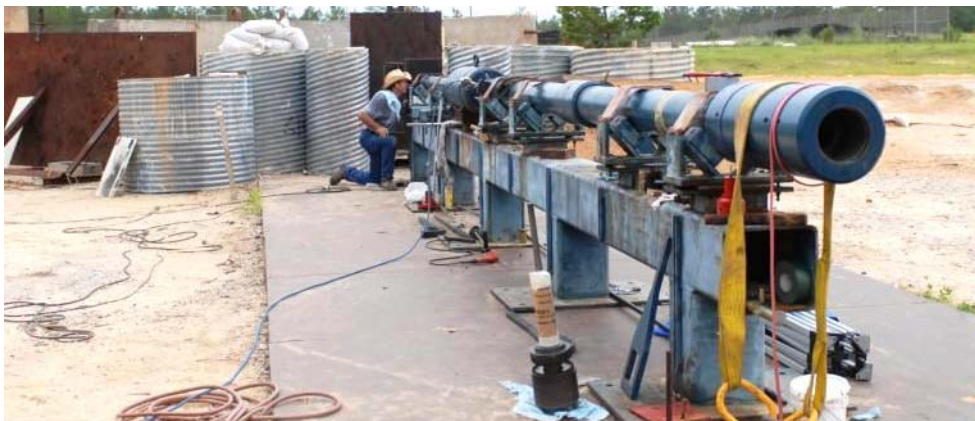
Figure 4. Two stage light gas gun used at AFRL Eglin AFB for fragment impact testing
