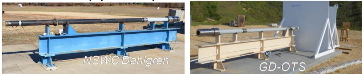
Figure 2 shows typical 40mm laboratory guns used for fragment impact testing.
