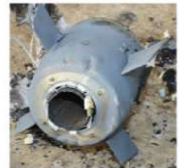
Type IV Response in SCO Trial – Ejected Aft Closure (Images Courtesy of MBDA UK)
