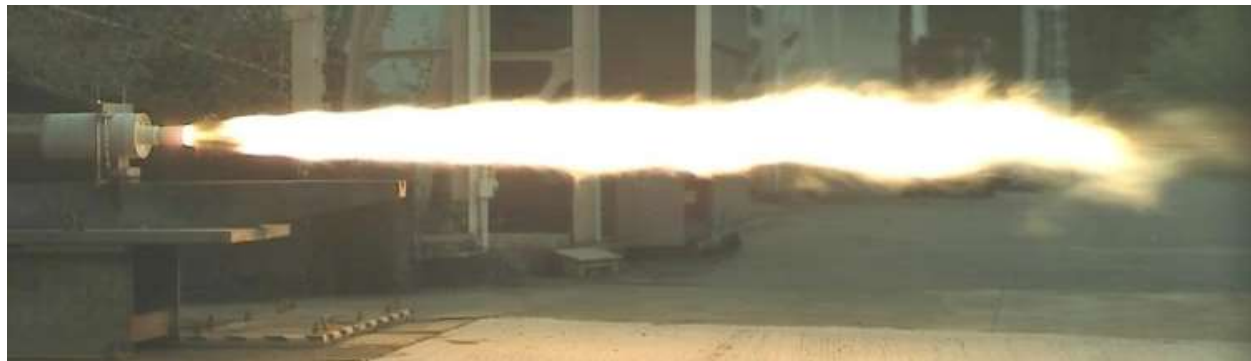
Vulcan Rocket Motor -46^{\circ}\text{C} Static Firing After Exposure To 98 days C2 Diurnal Cycling and 40 Thermal Shock Cycles
