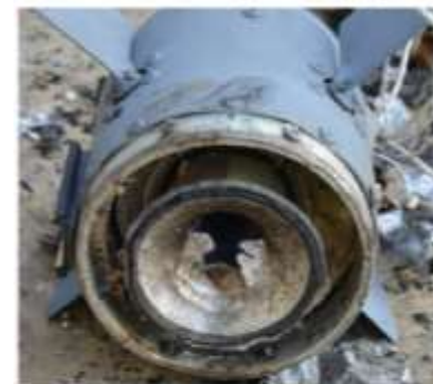
Type IV Response in SCO Trial – Ejected Aft Closure (Images Courtesy of MBDA UK)
