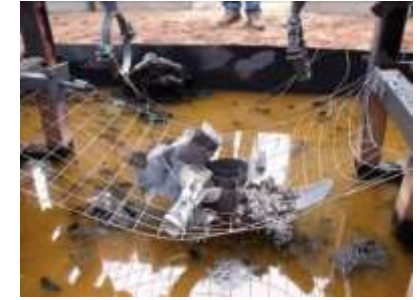
Vulcan Rocket Motor Type V IM Response to FCO; (Left) During The Fire, (Right) After Trial Condition
