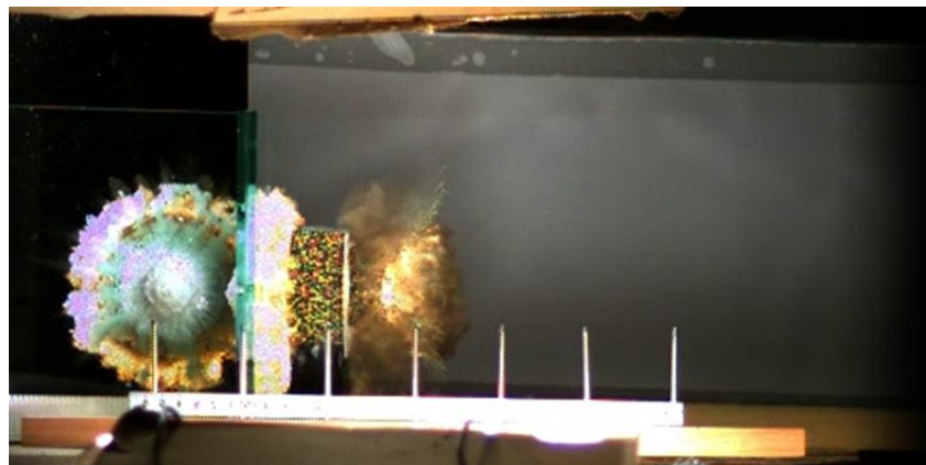
Figure 3: Phantom 7 image of the propellant burning response
