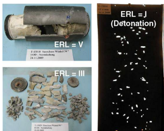
Fig. 8: Typical Explosive Reaction Levels (ERL) achieved during SCJ initiation tests.
