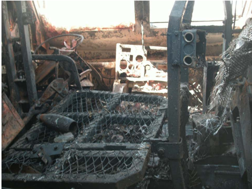
Figure 2. Interior view of the MRAP after the fire. An unexploded shell body from a M768 cartridge can be seen at the lower left.
