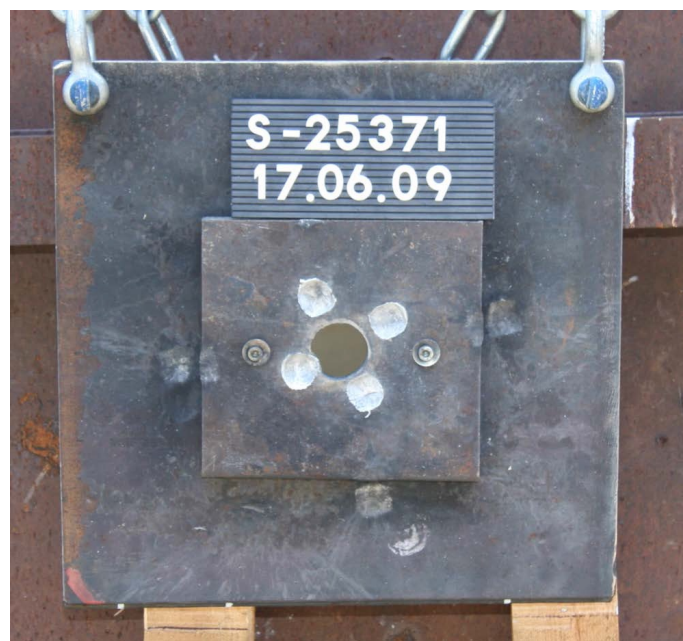
Figure 5: Stripper plate to stop the sabot (courtesy of TDW)
