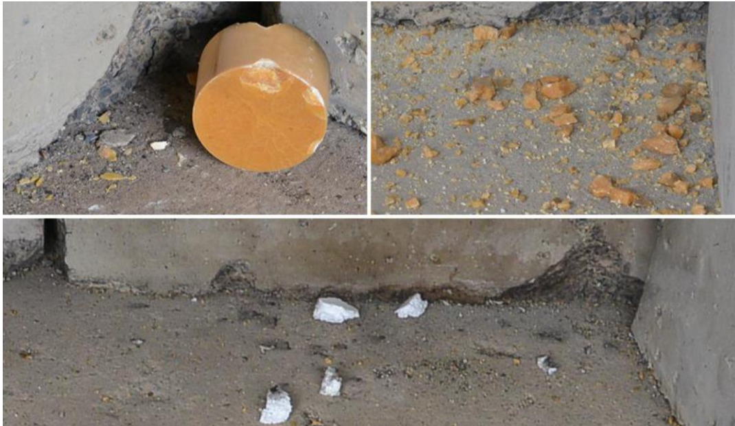
Figure 7: Structural responses of TNT. Clockwise from top left; Translation and relatively intact, large pieces and smaller debris, limited TNT debris (larger pieces identified)
