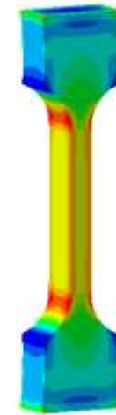
Tensile Specimen Modelled - (von Mises Stress)
