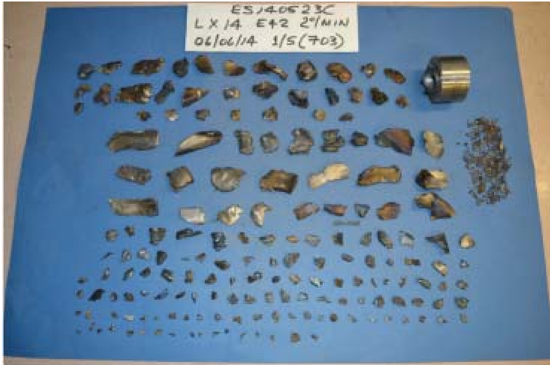
Figure 4 EMTAP 42 typical fragmentation for LX-14
