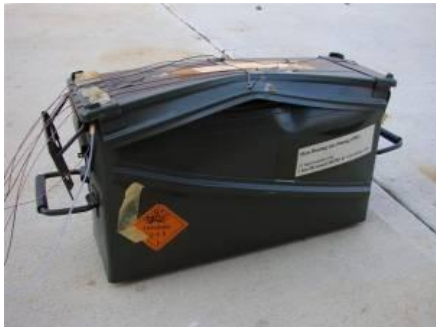
Figure 6: PA120 Box with 32 linked cartridges after test, in closed position and with lid removed
