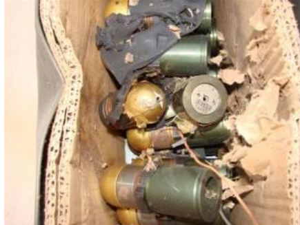
Figure 6: PA120 Box with 32 linked cartridges after test, in closed position and with lid removed
