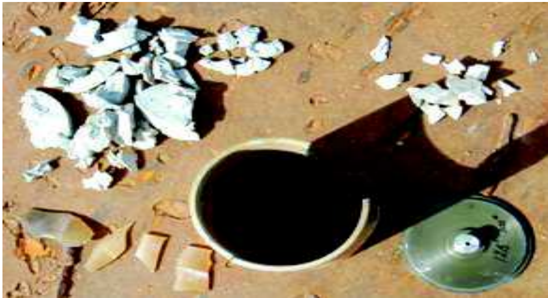
Typical type 4 reaction showing large chunks of un-reacted explosive
