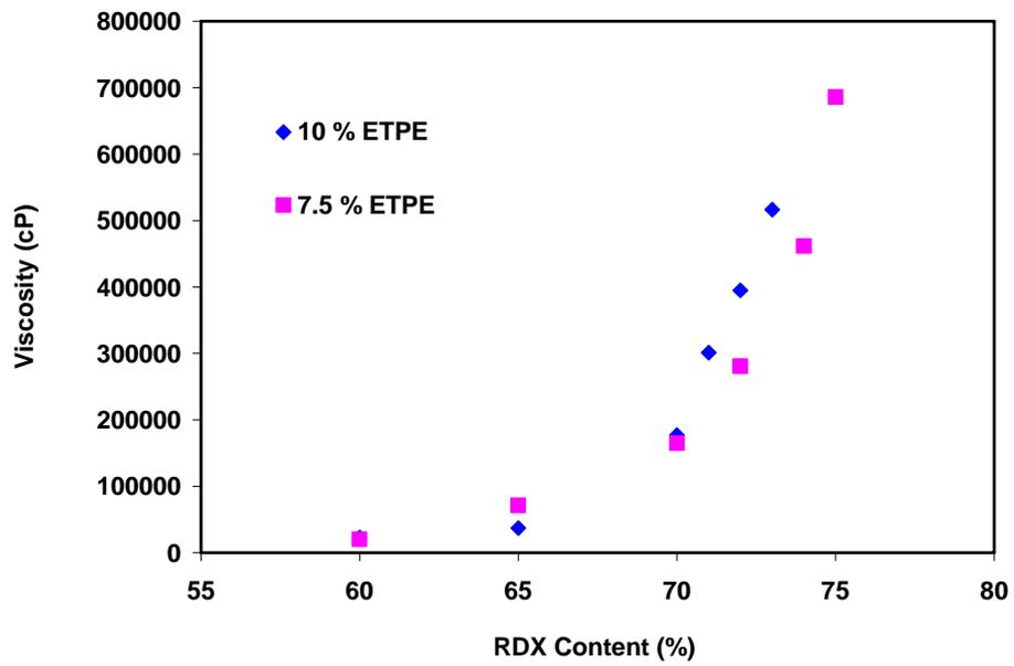
Figure 2: Viscosity as a function of RDX content in TNT/ETPE/RDX mixes.
