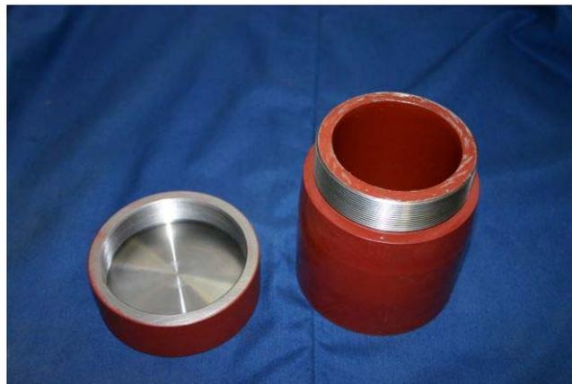
Figure 4: Test cylinder used in the bullet impact tests.
