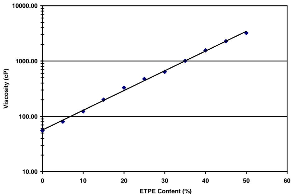
Figure 1: Viscosity of the TNT/ETPE mixture (measured at 95 °C).
