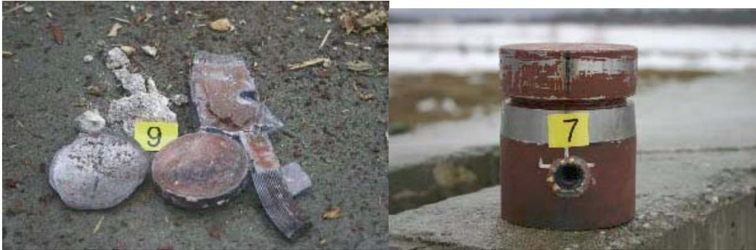
Figure 5: Bullet impact test results on HV-XRT 2. Left: violent reaction. Right: no reaction.
