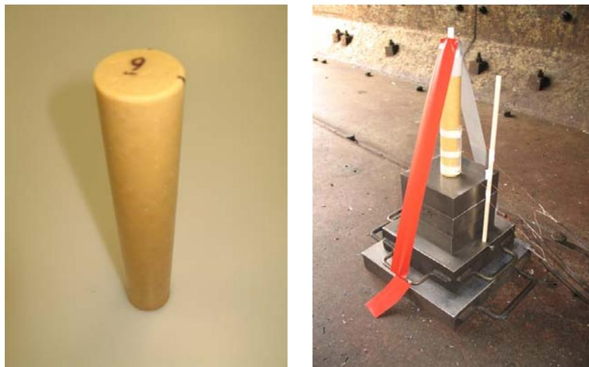
Figure 3: Left: cast cylinder of explosive for performance testing. Right: plate dent test coupled with velocity measurements.
