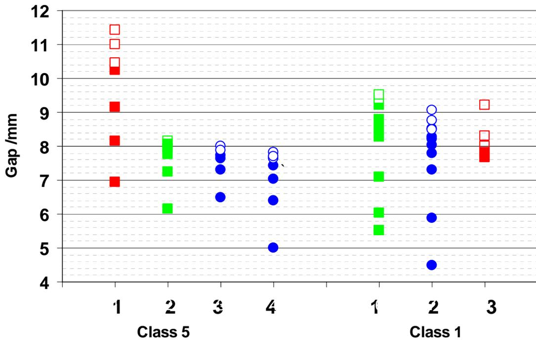
**Figure 2:** Gap test results for class 5 (10-30 μm) and class 1 (100-300 μm) batches. Open symbols represent “no go” events and filled symbols represent “go” events.
