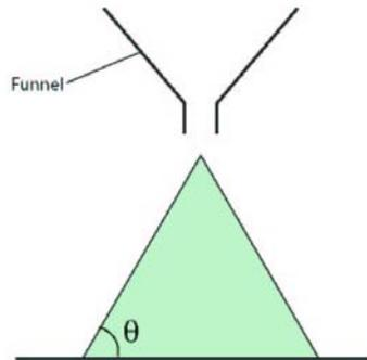
**Figure 5:** Schematic representation of the angle of repose. The material is poured through a funnel to form a conical pile and the angle between the horizontal and the side of the pile is measured.
