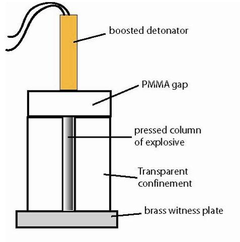
**Figure 1.** Diagram of the small-scale gap test. The charge was 5mm in diameter and 25mm long, contained within 25mm diameter PMMA.
