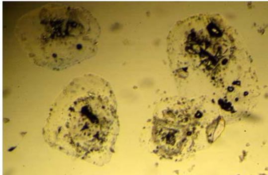
**Figure 4** ESEM and optical images of the medium-sized (class 1) material. The most sensitive (1) is shown at the top and the least sensitive (3) is at the bottom. The field of view of the optical images is 0.6mm wide.
