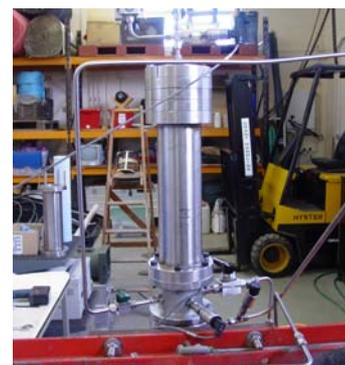
Figure 6: Gel expulsion test rig
