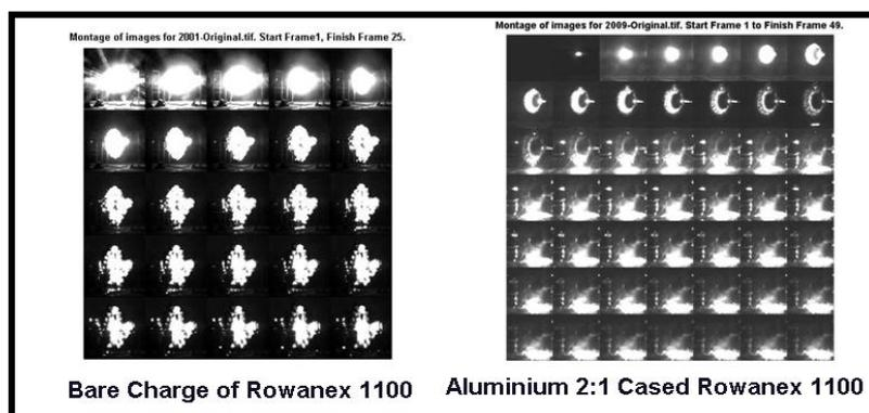
**Figure 6 – Typical Camera output showing ground effects following Aluminium case interaction with the arena floor.**
