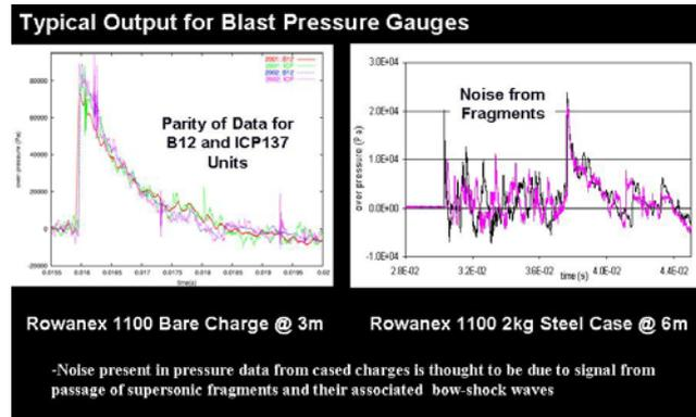
**Figure 4 – Typical output from Blast Pressure Gauges**
