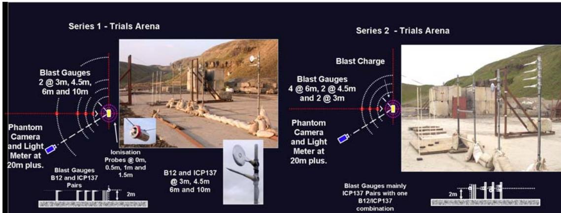
Figure 3 – Trials Arena for series 1 and 2 tests.
