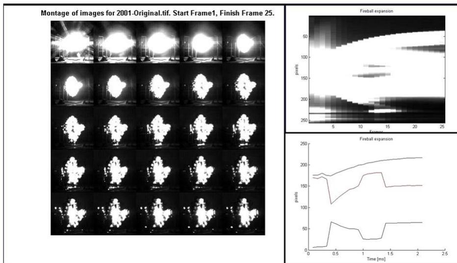
**Figure 8 – Automated tracking of Fireball Products using MATLAB.**
