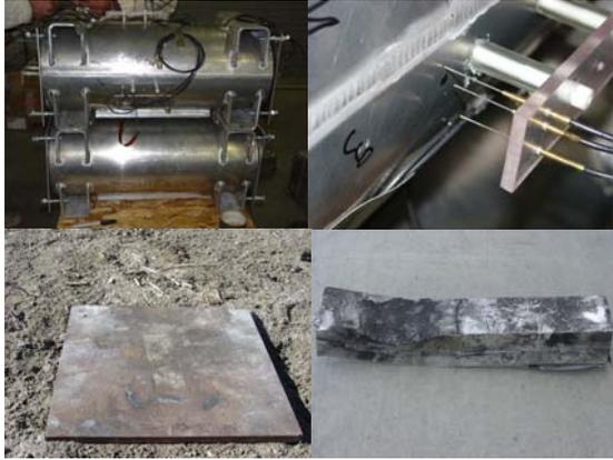
**Figure 7: Single Interrupter Test Configuration and Witness Plate**
