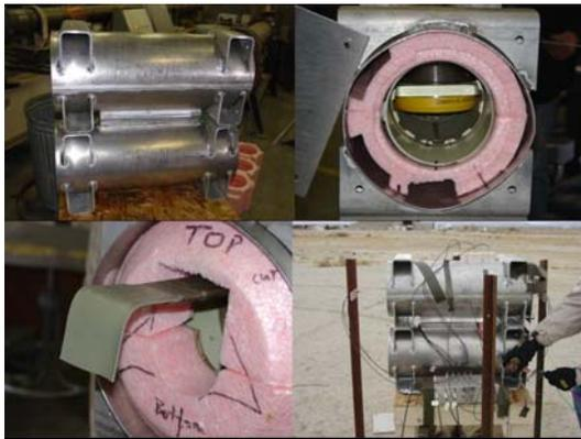
**Figure 4: Sympathetic Detonation Test Configuration**
