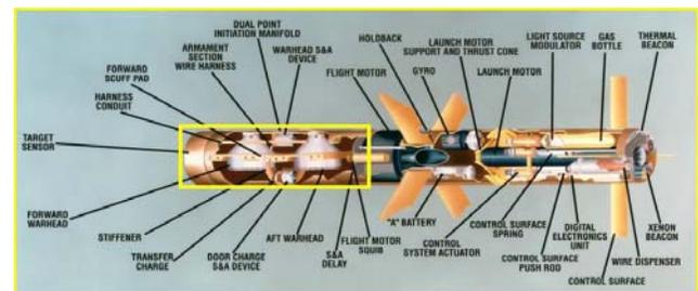
**Figure 2: TOW 2B Missile with Warhead section and palletized configuration**
