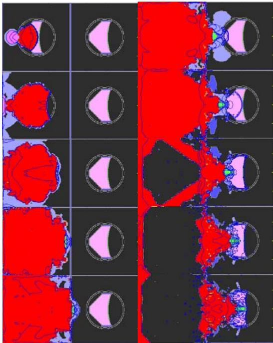
**Figure 3A & 3B: CHT Model Output Shows Pressure Level Below Acceptable Detonation Limits**
