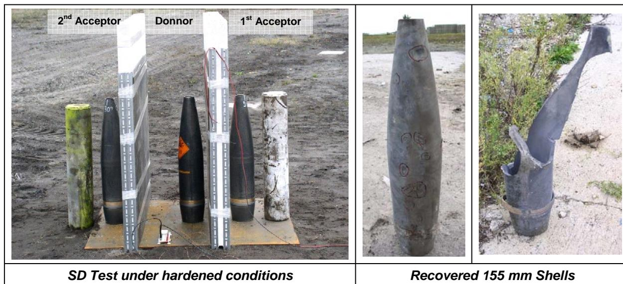
It is very interesting to note that the acceptors have not detonated even under stronger conditions. The closest acceptor has been torn and the other is pristine except the tracks of fragment impacts. Nevertheless, the projection distances can reach 150 m in open field due to effects of donor detonation. Using the pallets, these distances are shorter.
