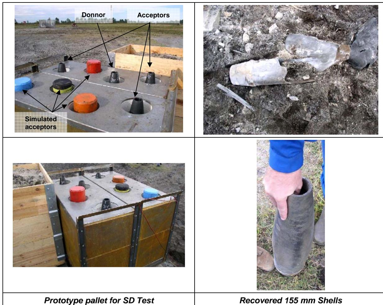
The results have shown the absence of sympathetic detonation in standard conditions between internal items and between pallets. The recovered acceptors are shown on the picture above. The nearest acceptor is partially torn, the two others are intact.
