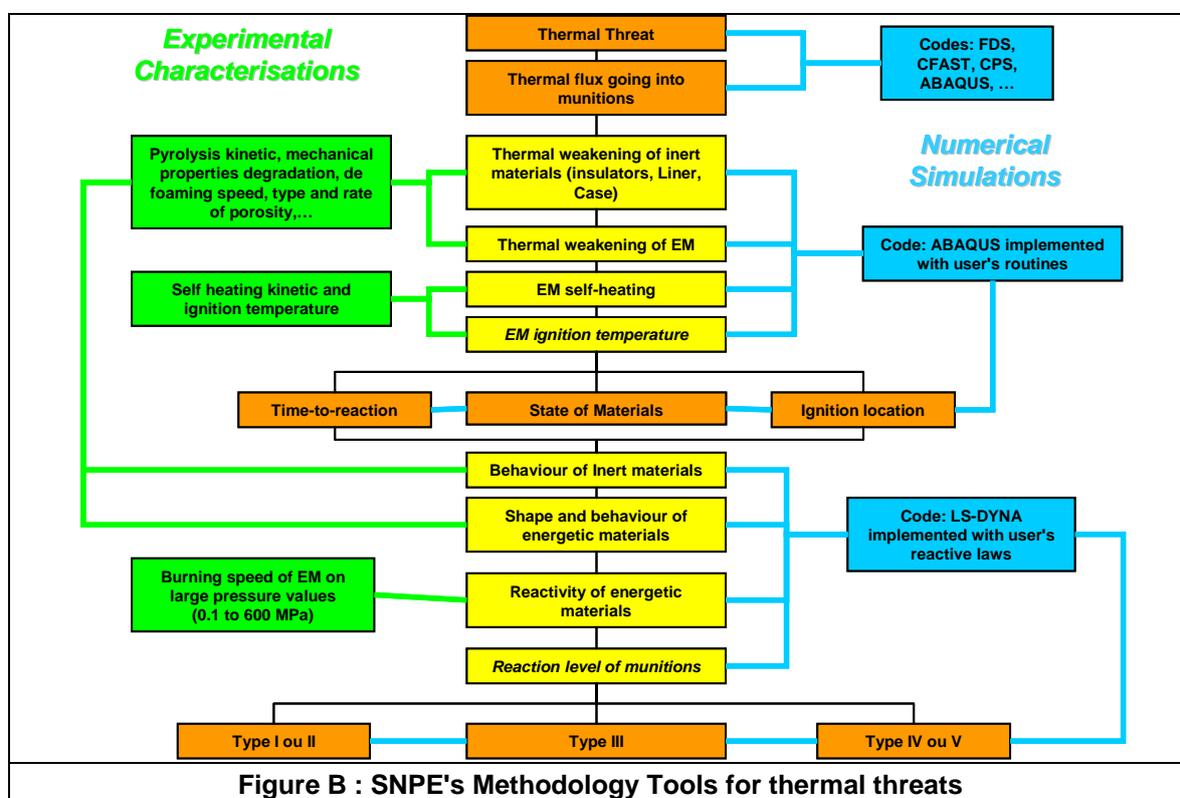
**Figure B : SNPE's Methodology Tools for thermal threats**
