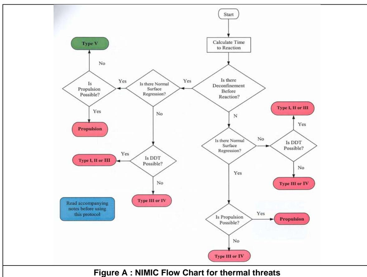
We can understand that behind every question several parameters must be taken into account. For example, question "is DDT possible?" forces to consider when an EM grain is damaged: - Which is its specific surface? - Which is its burning surface? - Which is pressure increasing rate? - Which is confinement pressure burst? - ... ..
