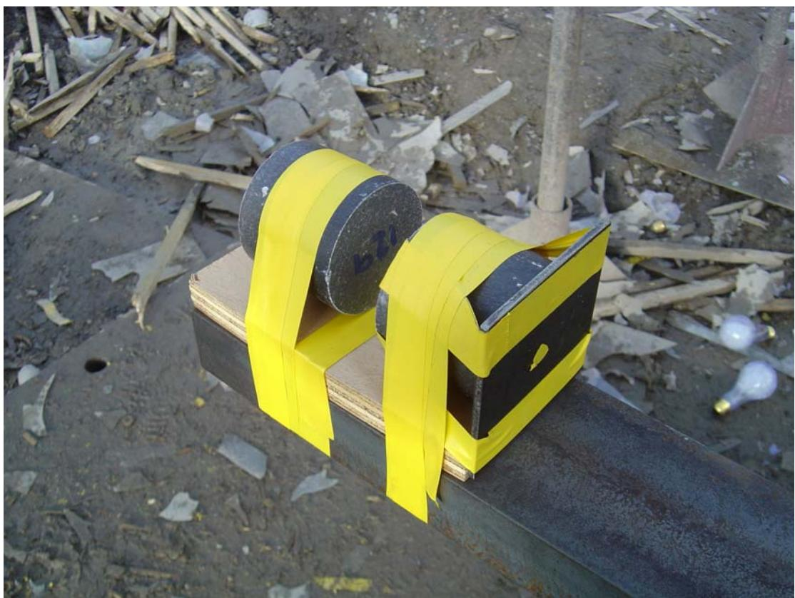
Figure 3. Experimental Set-Up for an XDT experiment with 2 ROWANEX 3000 charges and a steel cover plate.
