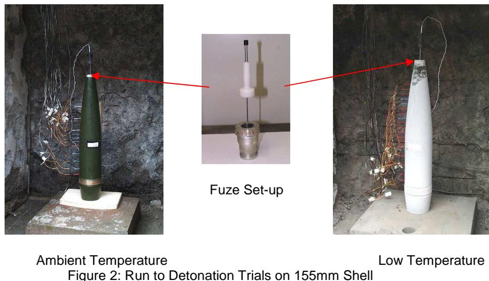
Land Systems has conducted a series of arena lethality trials on a full range of projectile natures (105mm HEIM, 105mm HEIMER, 155mm HEIM and 4.5" IM) using the lower output L116 fuze booster. These munitions have the same generic internal design (ROWANEX 1100 main charge and ROWANEX 3601 booster), and all firings have achieved successful detonation and fragmentation patterns.
