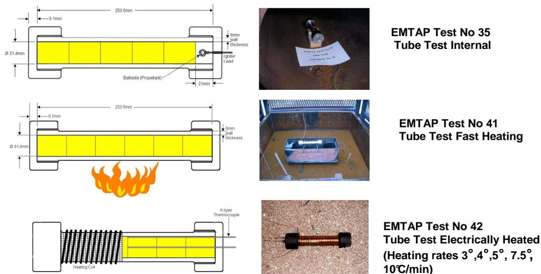
Figure 3: Three Variants of the the EMTAP Tube Tests
