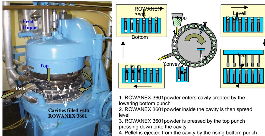
Figure 6: Rotary Pressing of ROWANEX 3601 Pellets
