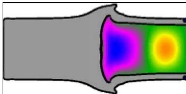
Figure 8: Simulation of the modified symmetrical Taylor test at 600m/s showing the stresses
