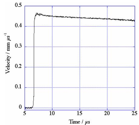
Figure 7: VISAR measurement from PBI impacted at 600m/s
