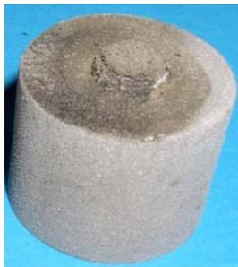
Figure 13: Reduced cavity sample post test
