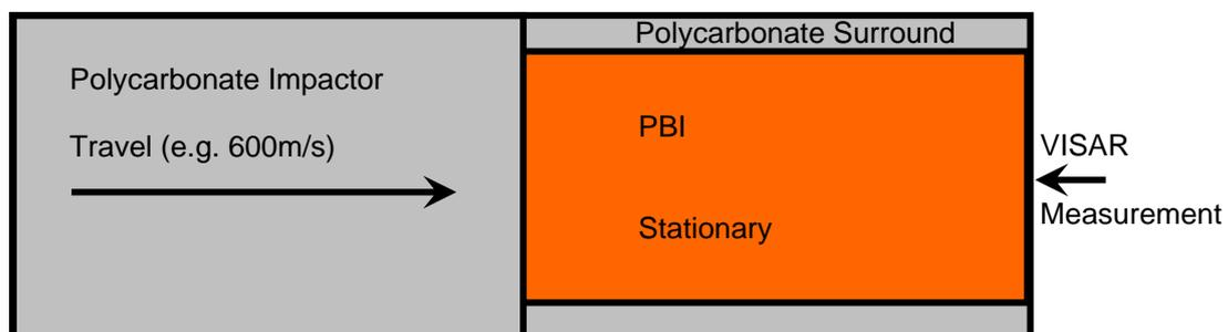
Figure 5: Experimental arrangement of the modified Taylor test
