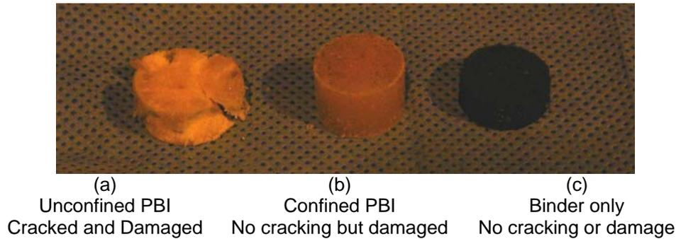
Figure 1: Examples of constitutive response – after quasi-static compression
