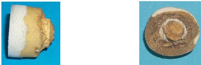
Figure 12: Sample post test with a change in confinement: set-back (L) set-forward (R)
