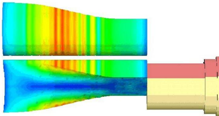
Figure 4: Stresses in the distorted energetic fill with a rifled barrel with a friction coefficient of 0.05
