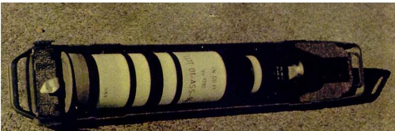
The logistic case is a GIAT 21 model. The individual case is composed of a part in high density polyethylene (PEHD-THP M) and a part in rigid moss.
