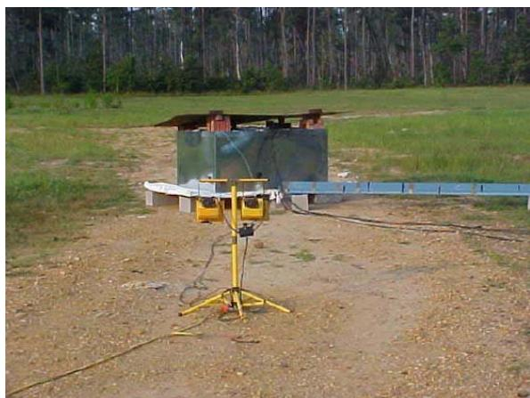
**Figure 4. Slow Cook-Off Test Setup**
