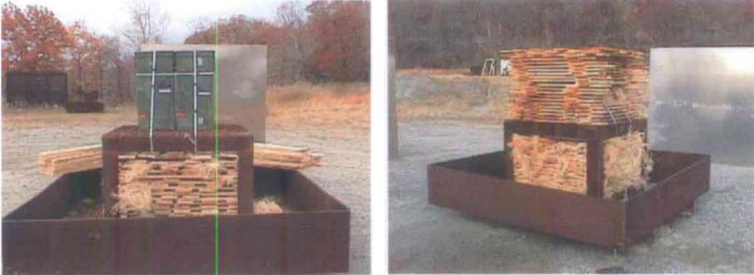
**Figure 7. External Fire/Fast Cook-Off Test Setup**
