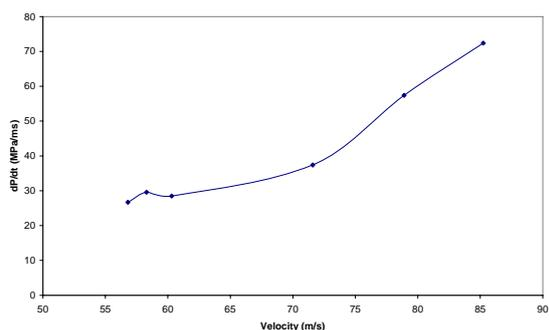
Figure 5. Pressure derivative as a function of the sample velocity in the Friability test.
