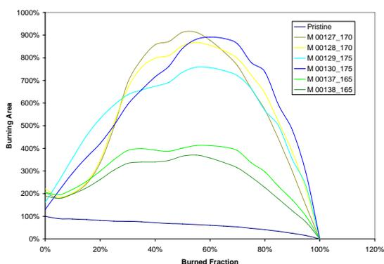
Figure 7. Burning area increase due to thermal damage of HMX-PBX samples.
