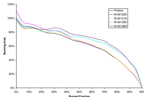
Figure 4. The calculated burning areas of the pristine, single and double cycle damaged HU45 at 20% compression.
