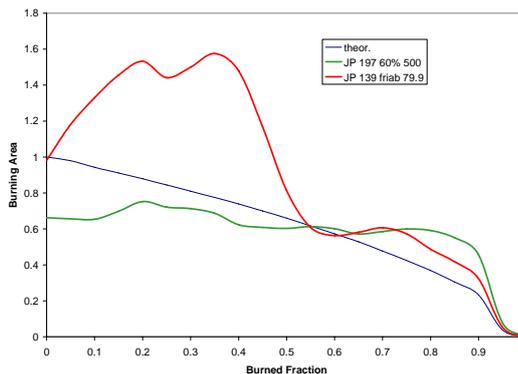
Figure 6. Comparison of the burning area of due to damage in the a gas gun experiment at 79.9m/s and a compression test at 500 mm/min up to 60% compression.
