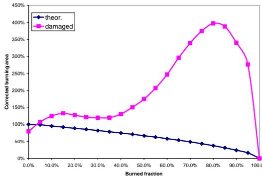
Figure 2. Burning area as a function of the burned fraction for a pristine and damaged sample.
