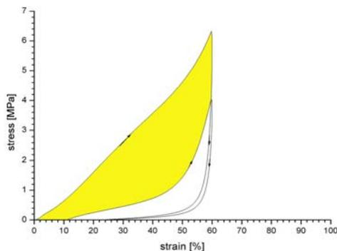
Figure 3. Area between two compression cycles, indicating the extend of damage.
