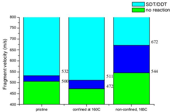
Figure 9. The impact sensitivity of HU 45 in pristine state, heated and confined state, heated-then-cooled and non-confined state. Impact with the Ø22 mm tungsten fragment.
