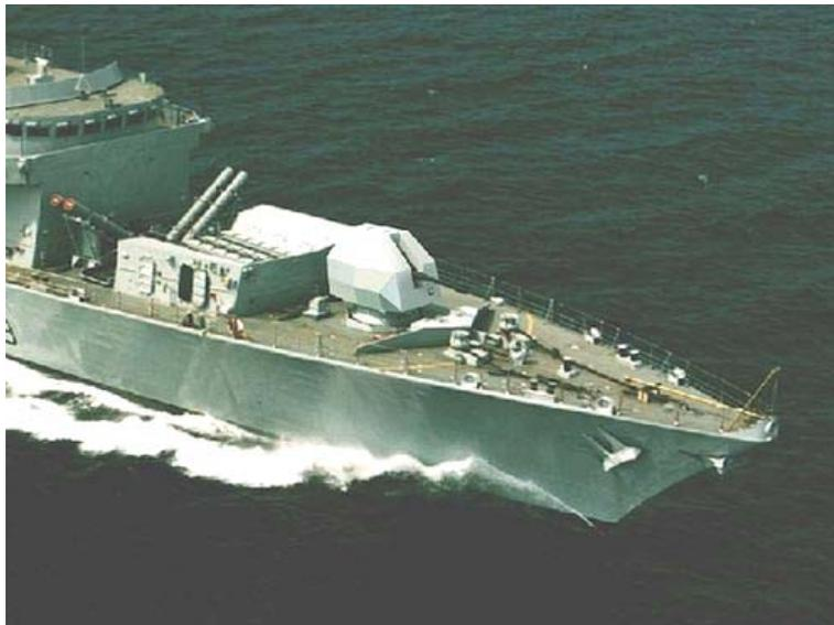
Figure 1 –4.5 Inch Mk 8 Mod 1 Gun fitted to a Type 23 frigate.
