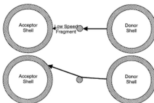
Figure 3 – Anti-Fraticide Bar showing its influence in reducing fragment impact into an acceptor.
