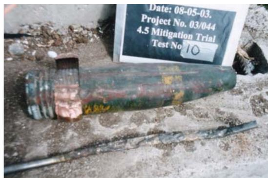
Figures 5 & 6 – Firing set up and recovered acceptor post firing showing markings from bar impact and deflected fragment strikes above the critical angle of perforation.
