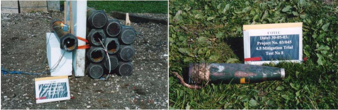
Figures 11 & 12 – Test set up for water barrier with 3 donors on right (initiated simultaneously) with 1 acceptor to the left. Fig 12 shows recovered acceptor showing no fragment impact markings and little casing compression due to blastwave loading.
