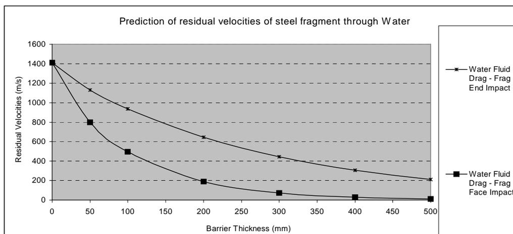
Figure 10 – Predictions for Unitised Barrier using Schonberg Projectile Penetration method. A comparison is made between fragment face impact with the larger presented area and fragment end impact, allowing for natural fragment formation.
