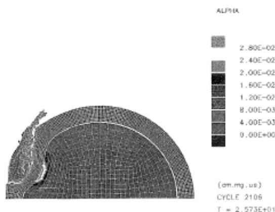
Figure 4 - Contour Plot for indirect impact of deflected fragment above critical attack angle.
