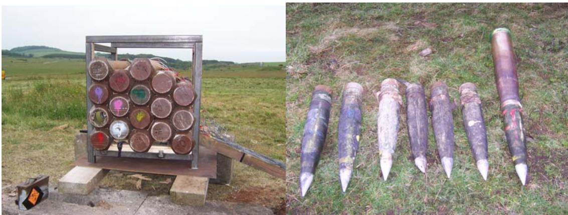
Figures 7 & 8 – End on Set up for stack tests. Donor is second from bottom on left column. 7 Acceptors surrounding and 9 ballasted containers are placed on the periphery. Right - 7 Recovered acceptor shell and cartridge post firing.
