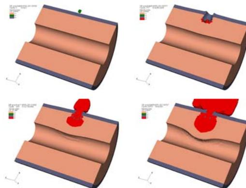
Figure 6. Impact Response at 6,000 fps (Time = 0, 80, 160, 320  $\mu$ s)
