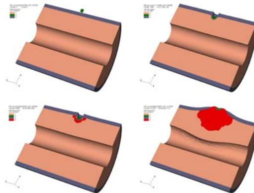
Figure 7. Impact Response at 3,280 fps (Time = 0, 130, 380, 633  $\mu$ s)
