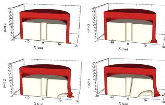
Figure 2. CTH Material Plots for Rocket Motor Surrogate at 12,000 fps
