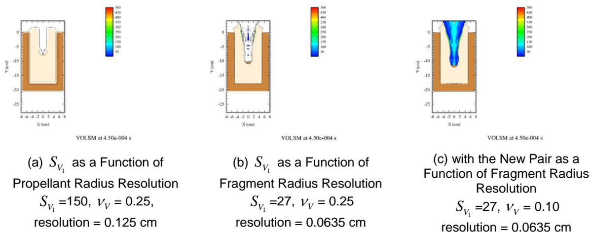
Figure 4. Volumetric Burn Corresponding to Fragment Impact into Bare Propellant
