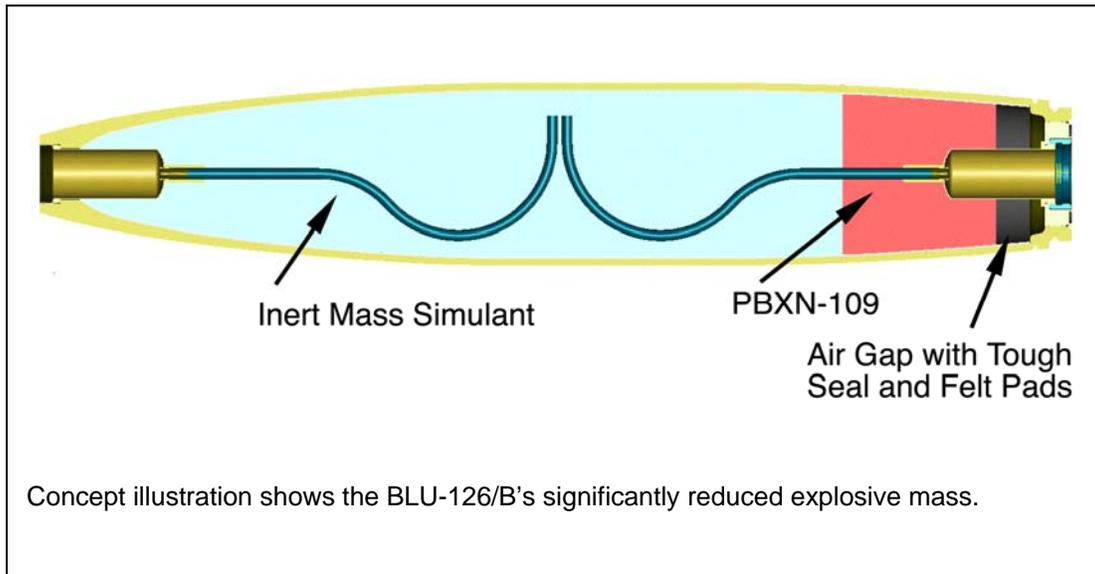
The proposed BLU-126/B design solution was developed under the following constraints:
