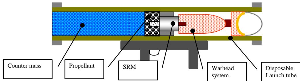
Figure 1– A schematic illustration of the AS shoulder launched rocket
