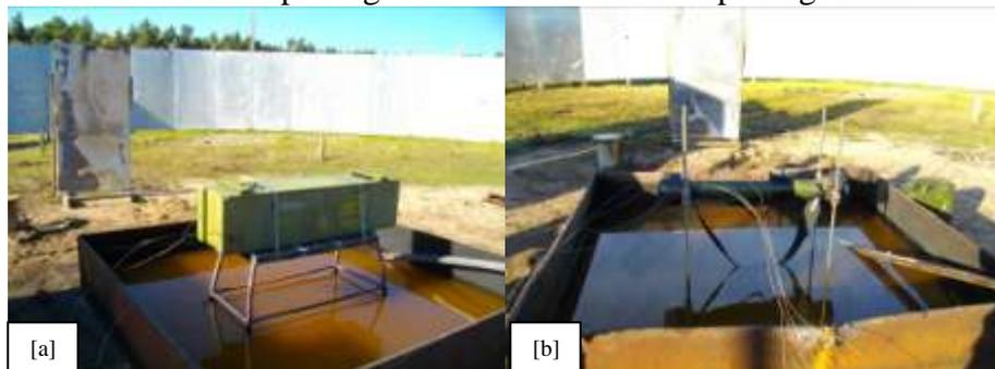
**Figure 10 – AUR Fast heating test setup for packaged [a] and unpackaged [b] configurations**
