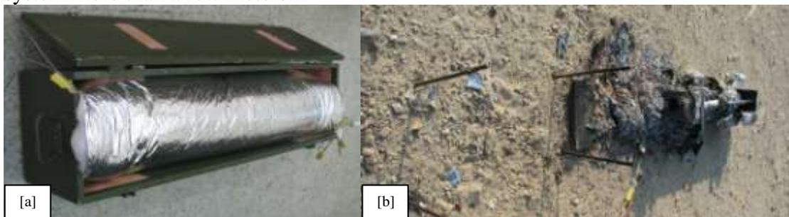
**Figure 8 – Propulsion system preliminary slow heating test setup [a] and results [b]**
