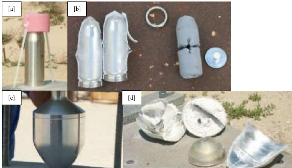
Figure 4 – Component level Bullet Attack test setup and results for FTB [a],[b] and BIC [c],[d]
