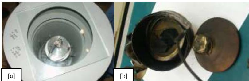
**Figure 7 – BIC component level slow heating test setup [a] and results [b]**
