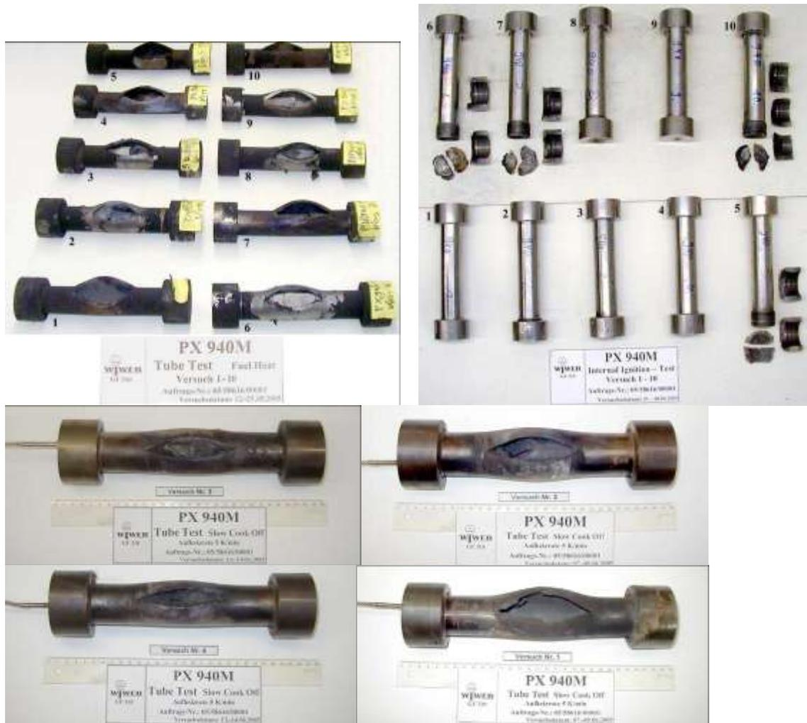
Figure 3 – PX940 Tube test results
