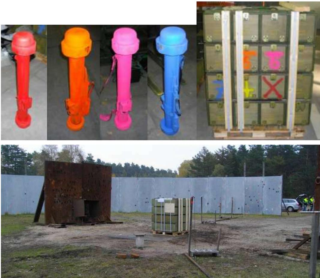
**Figure 11 – AUR sympathetic reaction test setup**
