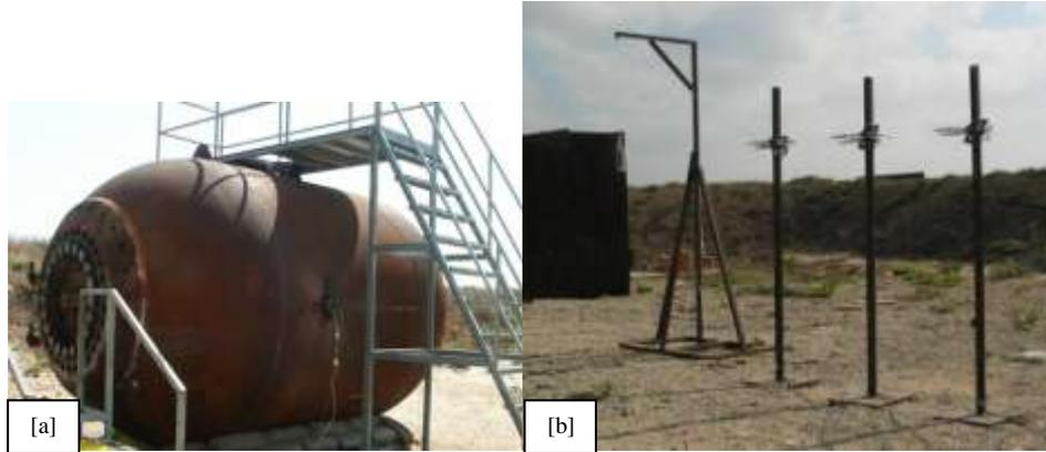
**Figure 2 – Explosive performance test setup [a] closed vessel [b] open field**
