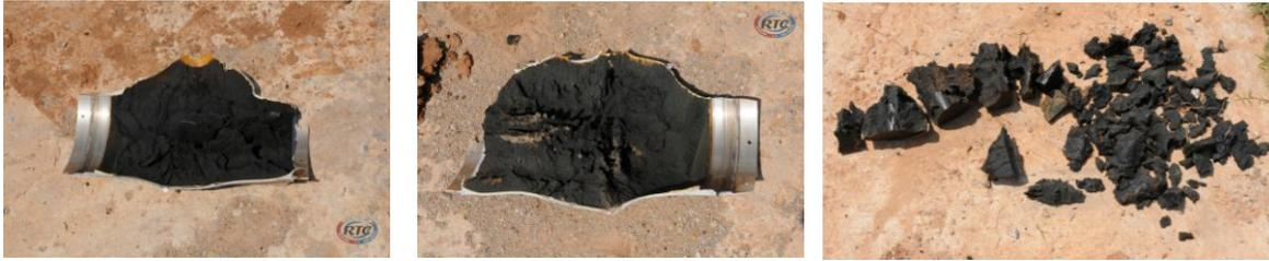
When tested in composite cases, the XLDB propellants demonstrated the ability to achieve no reaction to fragment impact velocities up to 2530 m/s (Figures 8 and 9). Additional testing is planned to explore variables in grain design and their impact on fragment impact performance.
