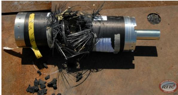
**Figure 9. Post-test Photo of 2530 m/s FI Test with Composite Case**
