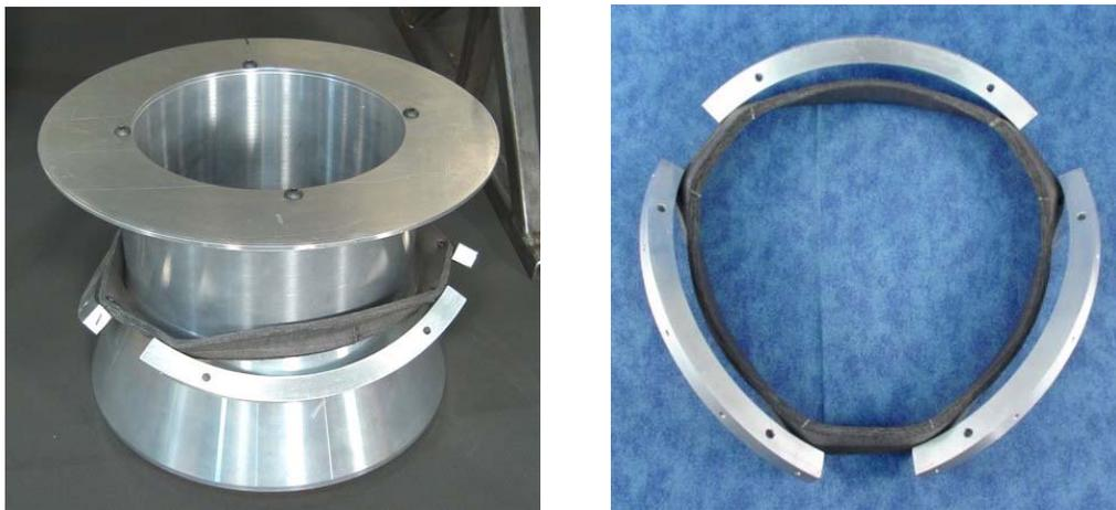
Figure 10. Released nozzle (left) and activated retaining ring (right)
