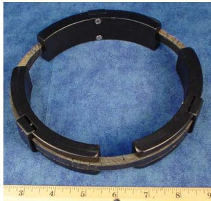
Figure 13. SMP retaining ring assembly
