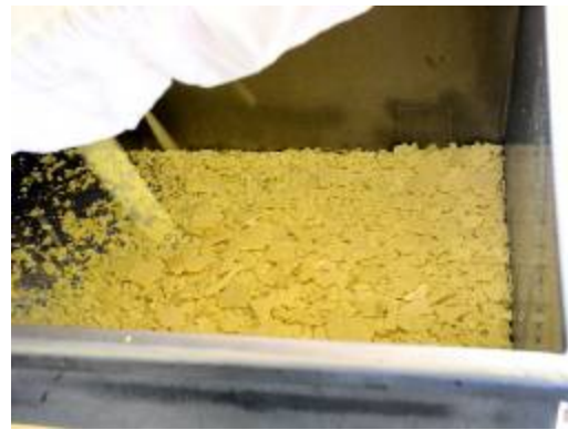
Figure 15 IMX-104 Flakes Collection in Nutsche
