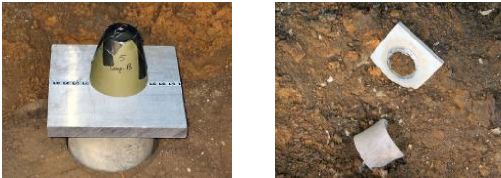
Figure 5 Initiation and Function Test of Composition B
