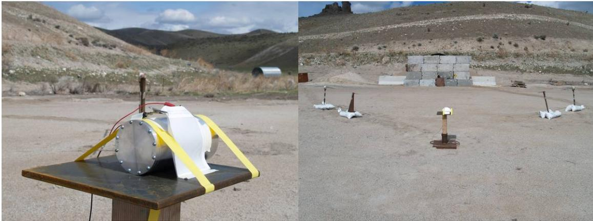
**Figure 2. The 3.2-inch Generic Shaped Charge Prepared for Bullet Impact Test**
