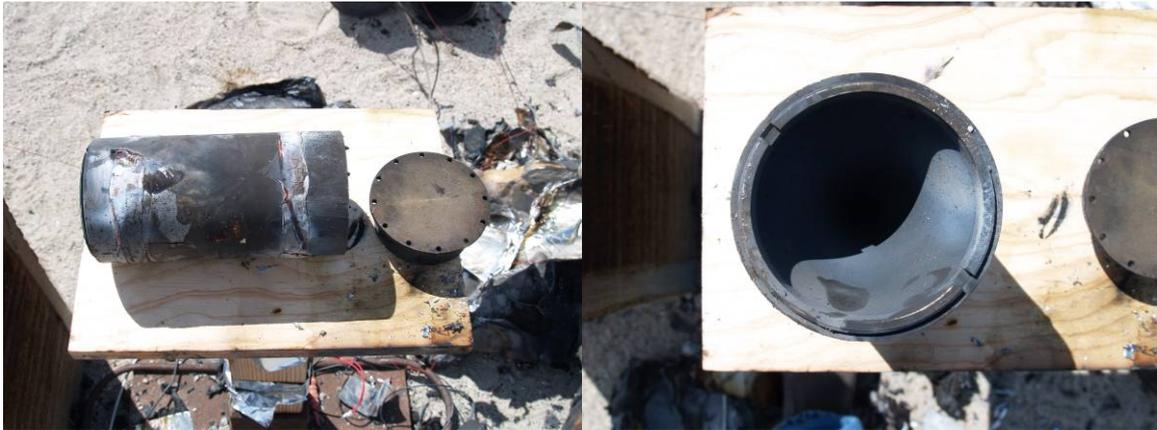
**Figure 6. Photographs of the Shaped Charge After the Cook-off Test (No damage to the liner or body was evident)**
