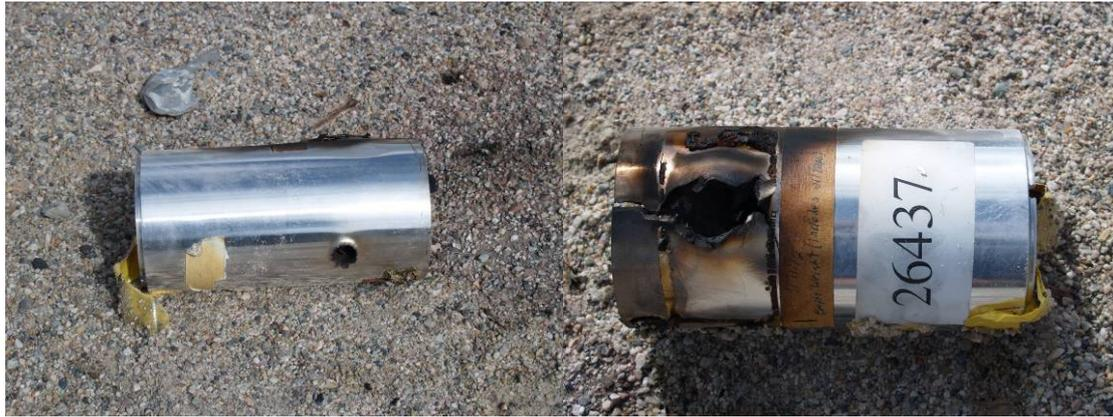
**Figure 3. Photographs Showing the Entrance and Exit Holes from the Bullet Impact Test**
