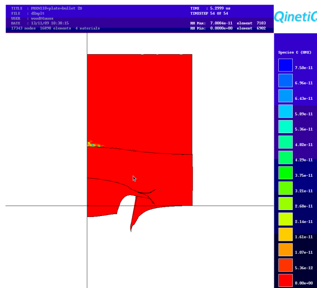
Figure 5: Final product concentration at 5.3µs after impact (very little reaction)
