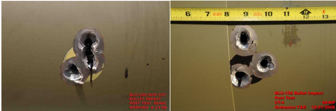
Figure 3. BLU-109 Bullet Impact Test Results
