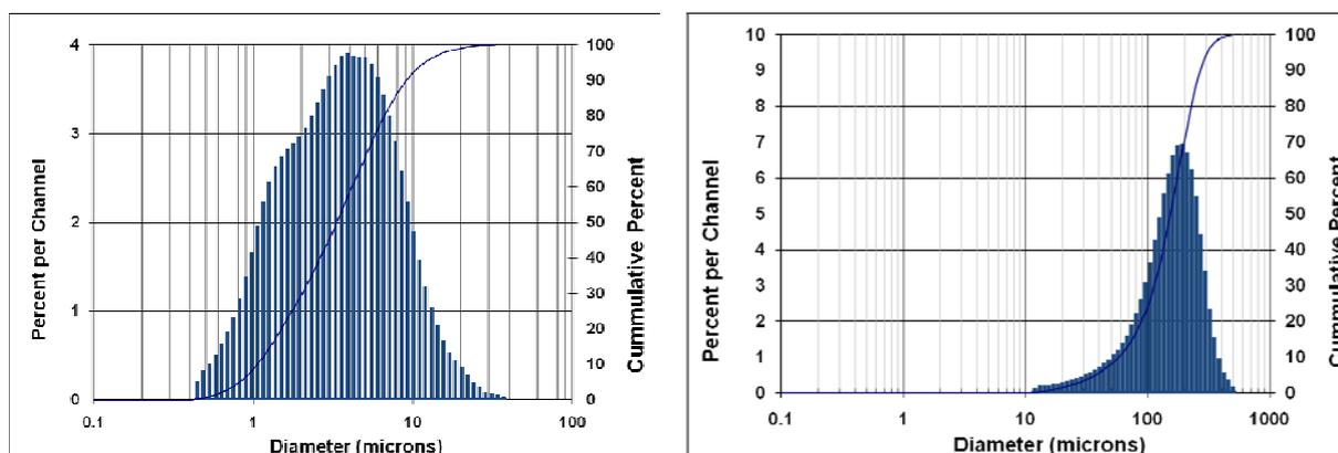
**Figure 2. Ground (l) and Unground (r) Particle Sizes of CL-20 Similar to Those Used in This Study**
