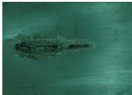
**Figure 8. Witness Plate After Critical Diameter Test Showing Detonation of All Samples of PAX-11 (smallest dent was made by 0.2-inch diameter charge)**
