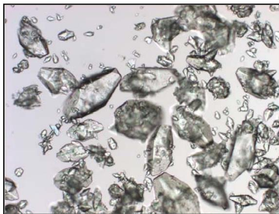
**Figure 1. Light Microscope Photograph of Unground CL-20 at 100X Magnification**
