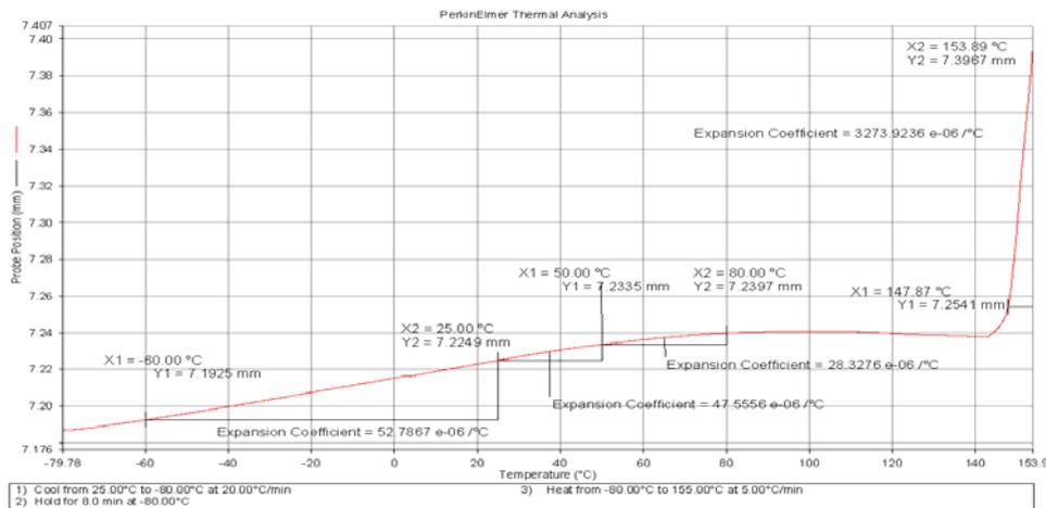
Figure 4. Plot of Growth Versus Temperature for PAX-11
