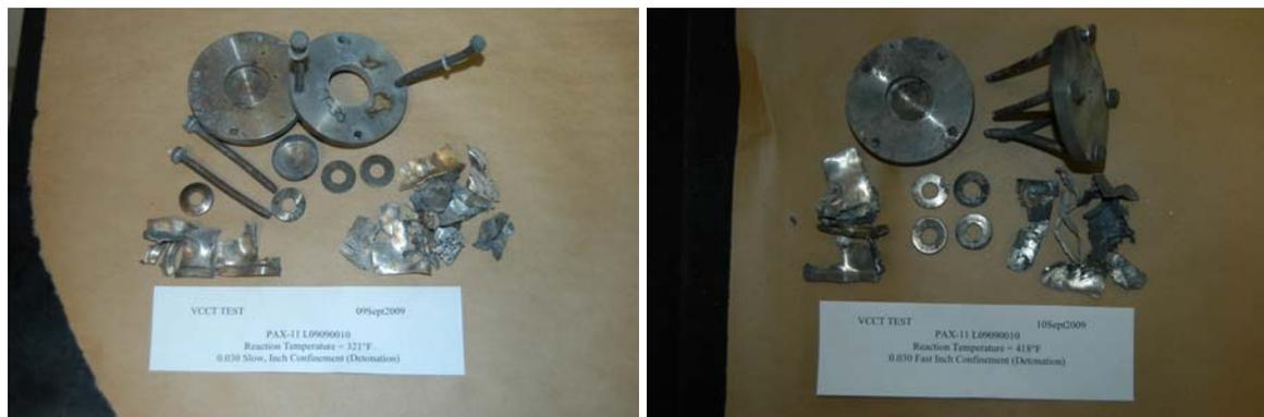
**Figure 3. Slow Cook-off (l) and Fast Cook-off (r) Tests at 0.03-inch Confinement**
