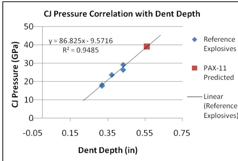
**Figure 7. Correlation of Dent Depth to CJ Pressure**
