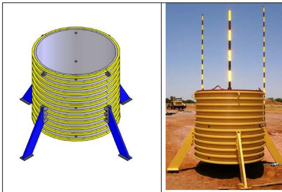
**Figure 1 Schematic representation (left) and a photograph (right) of the semi-confined VLIP apparatus**
