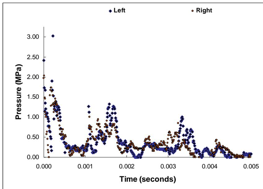
**Figure 5 Typical output of the overpressure sensors (two directly opposite sensors)**
