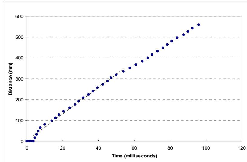
**Figure 2 Displacement versus time of the VLIP as measured off the high speed video recording (367kg plate and 300g charge)**
