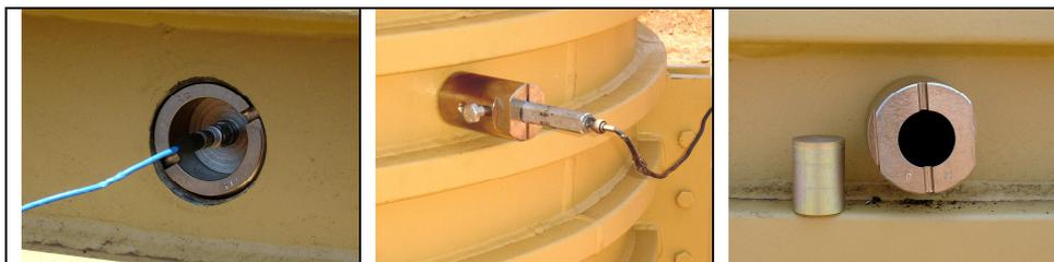
**Figure 3 (from left to right) Reflected pressure sensor, overpressure sensor fixture and momentum gauge**
