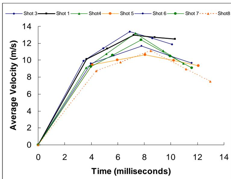
**Figure 7 Momentum gauge average velocity measurements**
