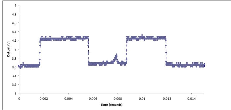
**Figure 4 Typical output of the momentum gauge measuring system**
