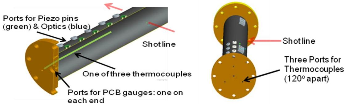
**Figure 3. Alternate Views of Baseline Test Fixture Showing Instrumentation Ports**
