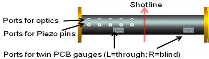
**Figure 2. Top View of Baseline Test Fixture Showing Instrumentation Ports**
