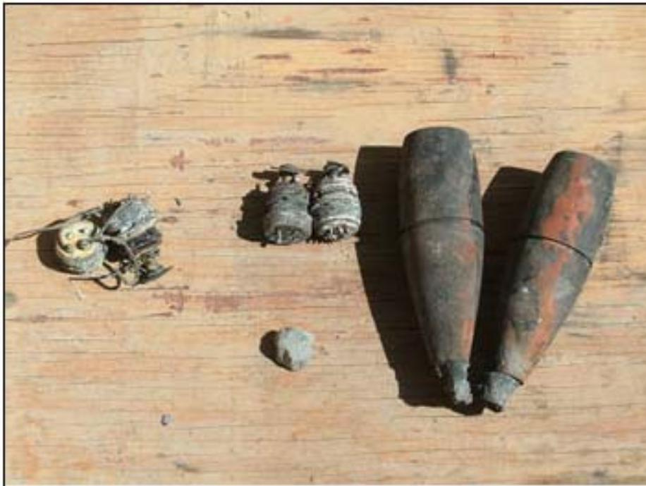
*Shell bodies and separated M783 fuzes from M768 cartridges recovered from the vehicle after the fire.*
