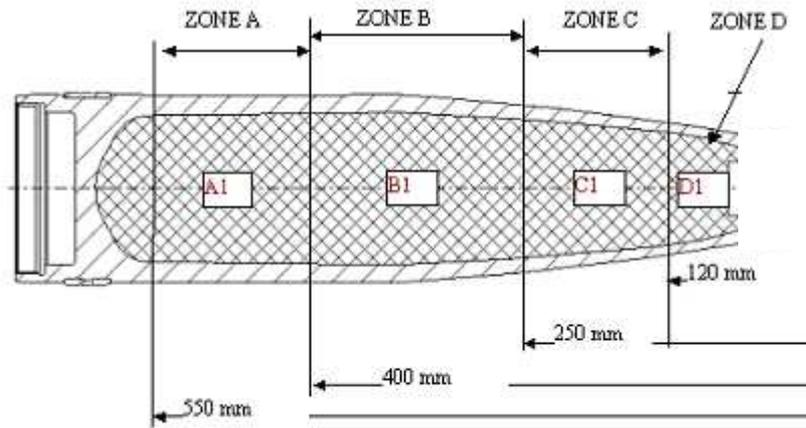
Figure 7: Strength and chemical XF® block samples – localisation
