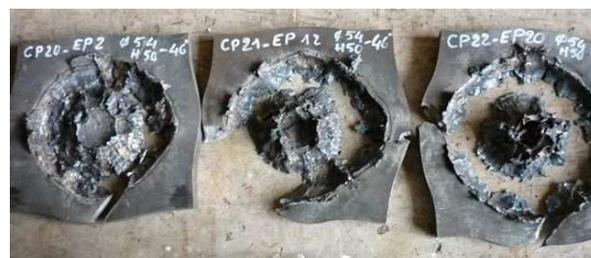
Figure 11: Recovery of the witness plates, test at -46°C
