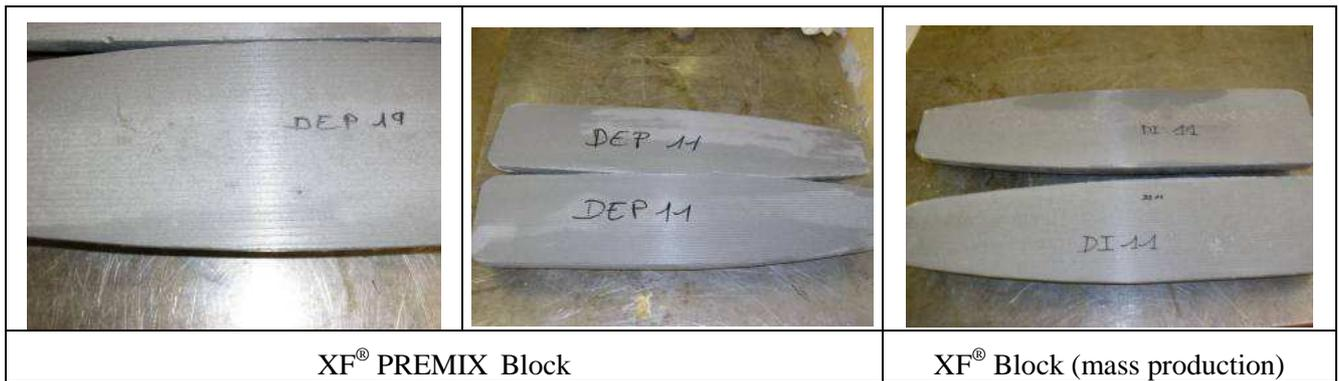
Figure 8: View of XF® PREMIX blocks after cutting
