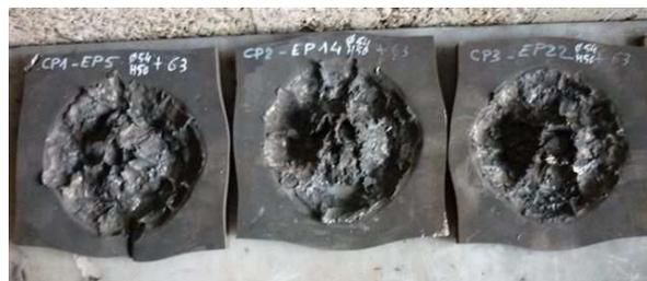
Figure 10: Recovery of the witness plates, test at +63°C
