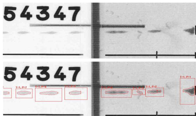
Measuring the  $V^2d$  is not easy or trivial. It is done through X-ray pictures (e.g. Figures 4 or 7). A grey scale value has to be defined to determine where the Shaped Charge jet diameter “ends”. Experiments with different grey scales gave different diameters by almost a factor of two. Also the measuring of the jet velocity behind a steel barrier P is not trivial and can be a source of additional scattering - exacerbated by the squaring of the velocity.
