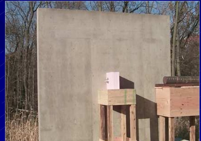
Concrete wall 10' wide, 10' tall 8" thick, reinforced with double steel rebar
