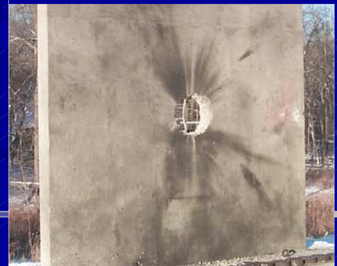
Concrete wall 10' wide, 10' tall 8" thick, reinforced with double steel rebar
