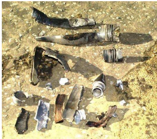
RDX/TNT 60/40 Fill with Debrix 18AS Booster
