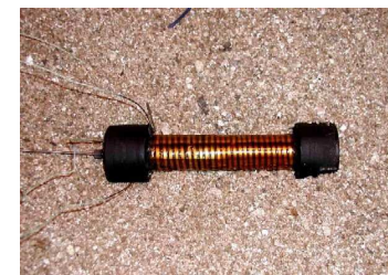
EMTAP Test No 42 Tube Test Electrically Heated (Heating rates 3°, 4°, 5°, 7.5°, 10°C/min)
