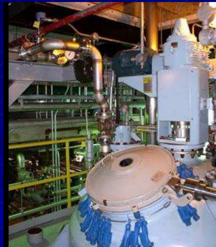
2,000 Gallon Glass-lined Reactor
