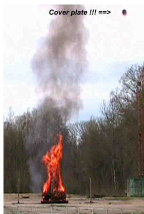
FIGURE 4: UN 6c test 3 liters of water in 220 liters barrels
