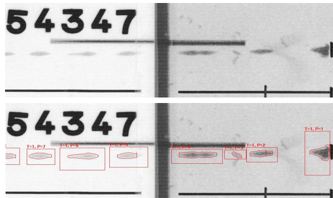
Figure 5: Measurement of SCJ particles from a X-ray pictures or a rotating mirror camera (MBDA TDW)
