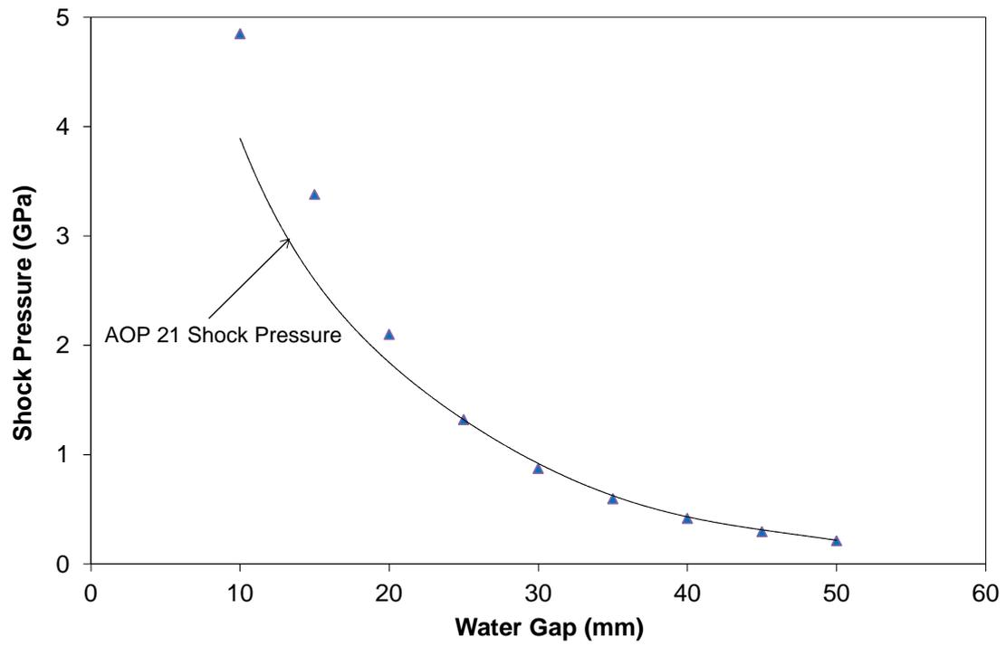
Figure 1; Curve of Shock Pressure against Water Gap.
