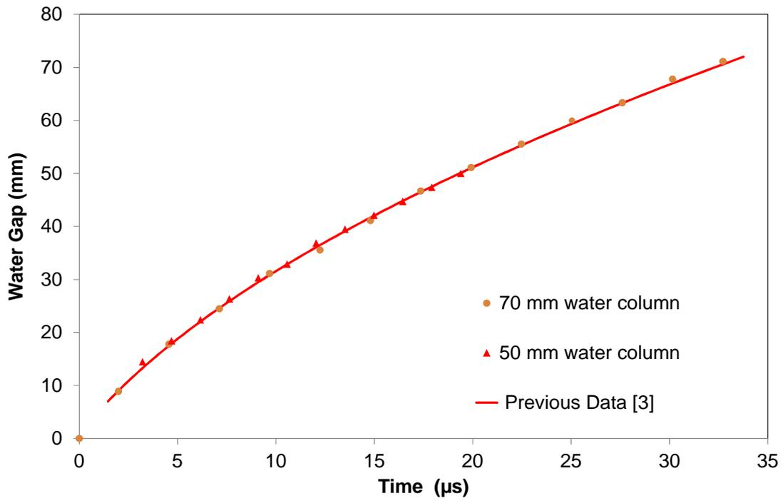
Figure 5; Comparison of high speed video for 70 mm and 50 mm water column and data reported previously [3].
