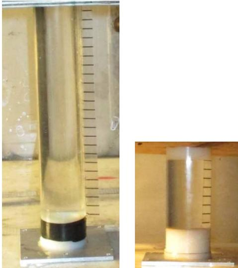
Figure 2; 240 mm and 75 mm water gap tests prior to firing.
