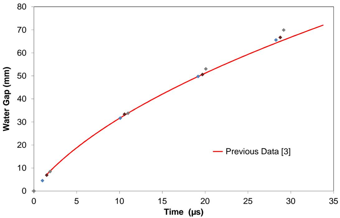
Figure 4; Comparison of high speed video for 250 mm water column and data reported previously [3].
