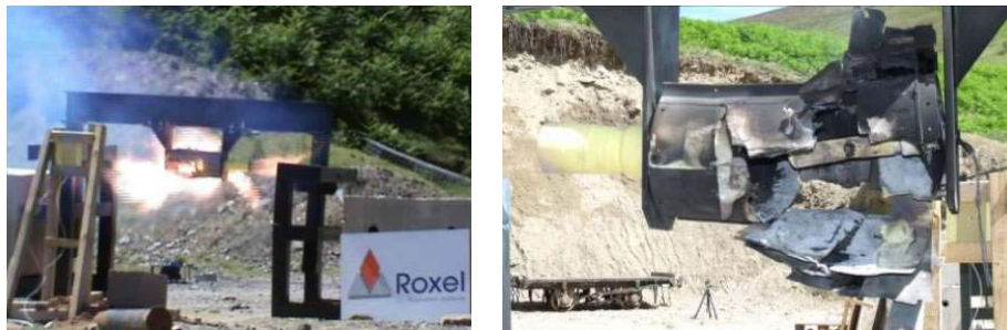
Vulcan Rocket Motor Type V IM Response to Bullet Impact; (Left) During Reaction, (Right) After Trial Condition
