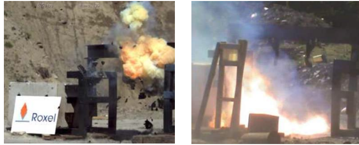
Vulcan Rocket Motor Type IV IM Response to Fragment Impact; (Left) Initial Impact, (Right) Subsequent Burning Response
