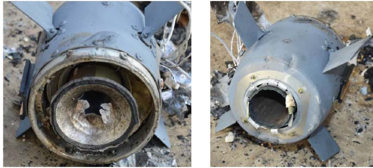
Type IV Response in Slow Cook Off Trial – Ejected Aft Closure (Images Courtesy of MBDA UK)
