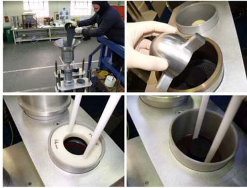
Staged Powder Filling and Consolidation During Casting Process
