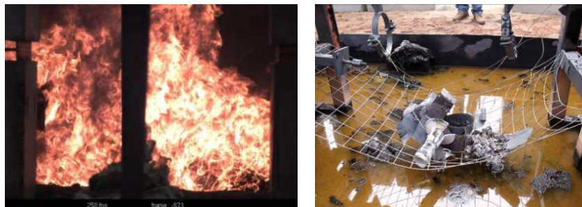
Vulcan Rocket Motor Type V IM Response to Fast Cook Off; (Left) During The Fire, (Right) After Trial Condition
