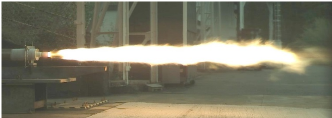
Vulcan Rocket Motor -46°C Static Firing After Exposure To 98 days C2 Diurnal Cycling and 40 Thermal Shock Cycles
