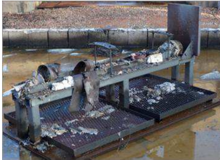
Figure 9: Image of Brimstone 2 system post IM Fast Heating trial
