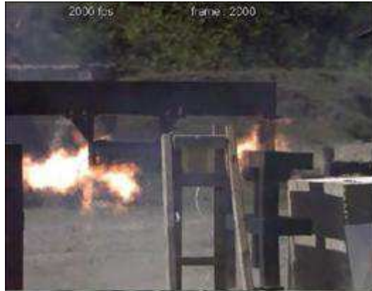
Figure 13: Vulcan Rocket Motor 1 second after Bullet Attack
