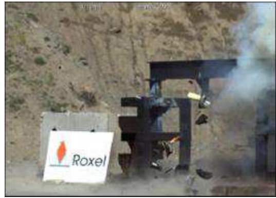
Figure 14 & 15: Rocket Motor Fragment Impact alternative velocity. Left image 3 ms after impact Right image 500 ms after impact
