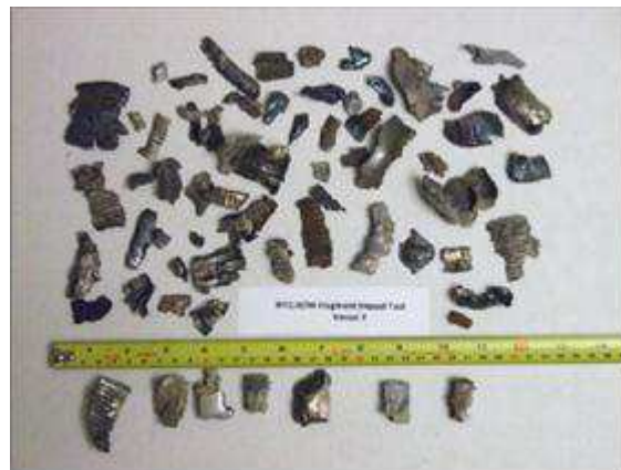
Figure 3 & 4: Response of SRS 142/F65(D3) to Fragment Impact 1911 m/s
