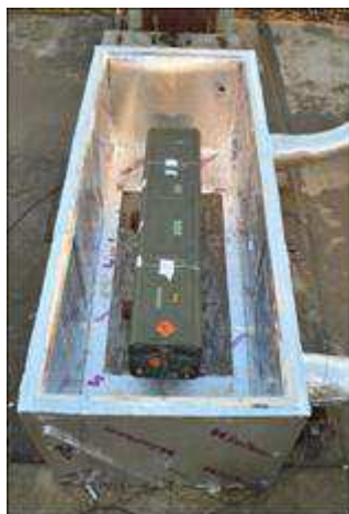
Figure 10: Packaged Brimstone 2 within Slow Heating oven
