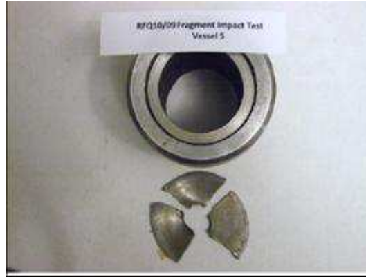
Figure 1 & 2: Response of SRS 142/F65(D3) to Fragment Impact 1848 m/s
