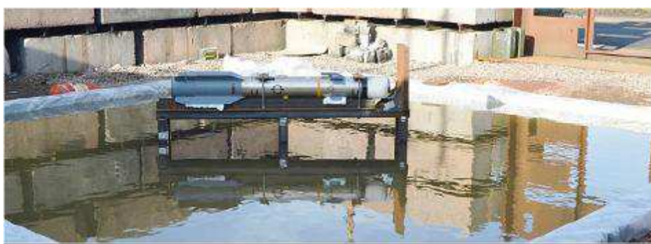
Figure 8: Brimstone 2 system prior to the IM Fast Heating trial.
