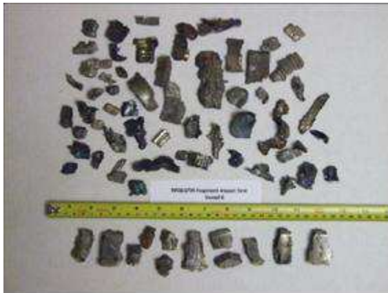
Figure 3 & 4: Response of SRS 142/F65(D3) to Fragment Impact 1911 m/s
