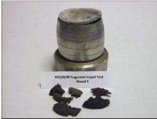
Figure 1 & 2: Response of SRS 142/F65(D3) to Fragment Impact 1848 m/s
