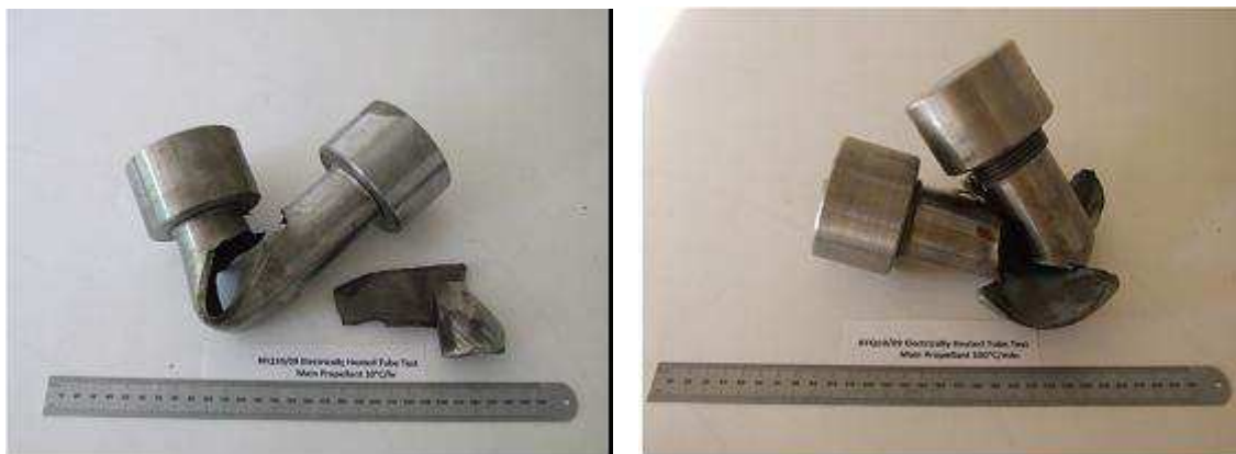
Figure 6 & 7: Response of SRS 142/F65(D3) to EMTAP 42 at 10°C/hour and 100°C/minute.
