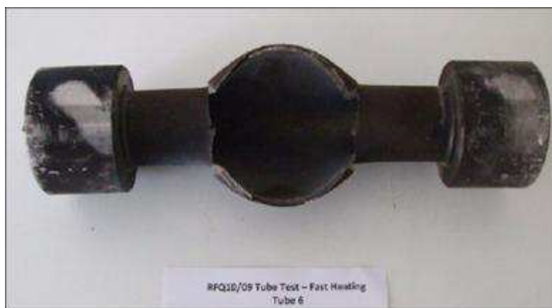
Figure 5: Response of SRS 142/F65(D3) to EMTAP 41 Fast Heating test.
