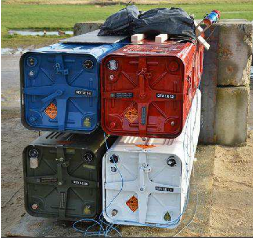
Figure 17: Sympathetic Reaction trial setup. Red live donor; Blue and White live acceptors; Green mass representative inert.
