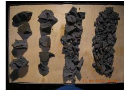
FI : Fragments of propellant & mock up metallic structure
