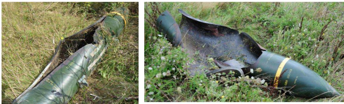
Figure 9. Reaction of two BLU-109 to heavy fragment impact
