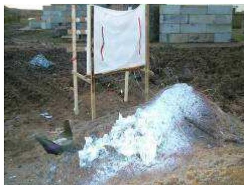
Figure 7. Violent mechanical break up and burnt out remains of 250 kg GP Bombs.
