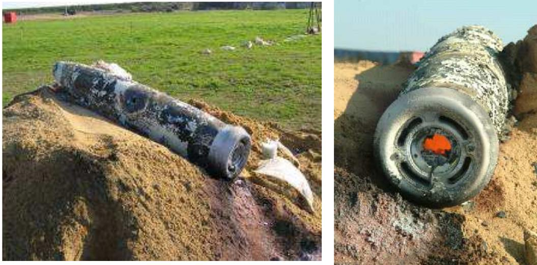
Figure 1. Burnt out Paveway IV after NATO IM 14.3mm fragment impact.
