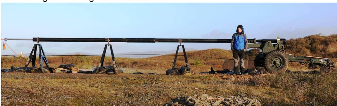
Figure 6. 10 m long 40 mm smooth bore gun
