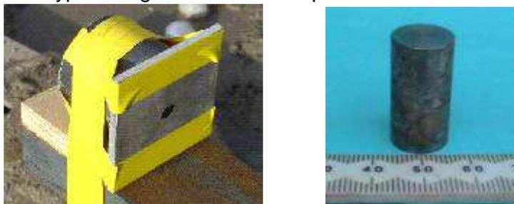
Figure 2. Fragment Attack set up and 13.15mm Fragment
