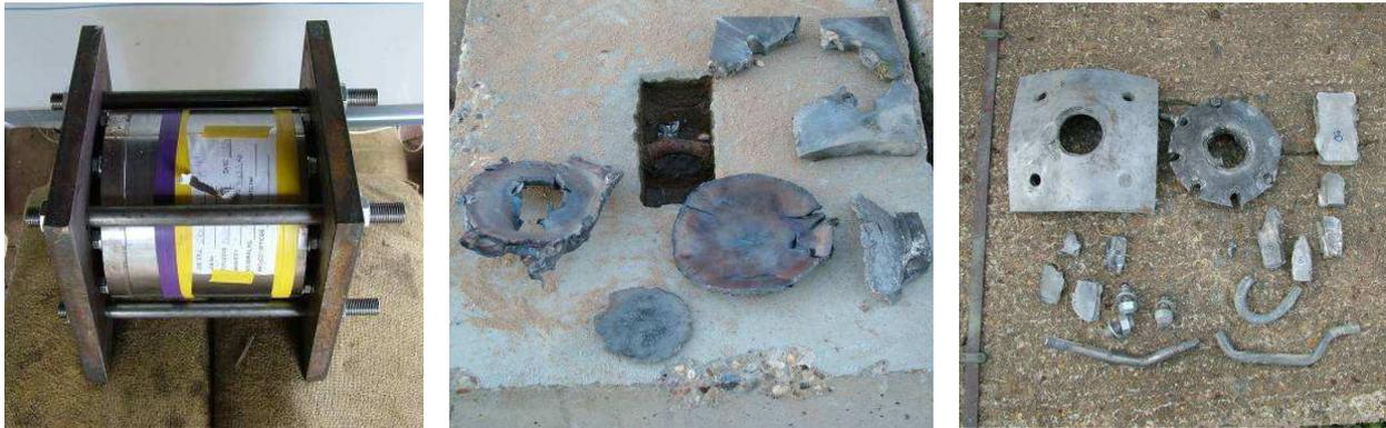
Figure 5. High confinement vessel, a detonation and suspected partial detonation.
