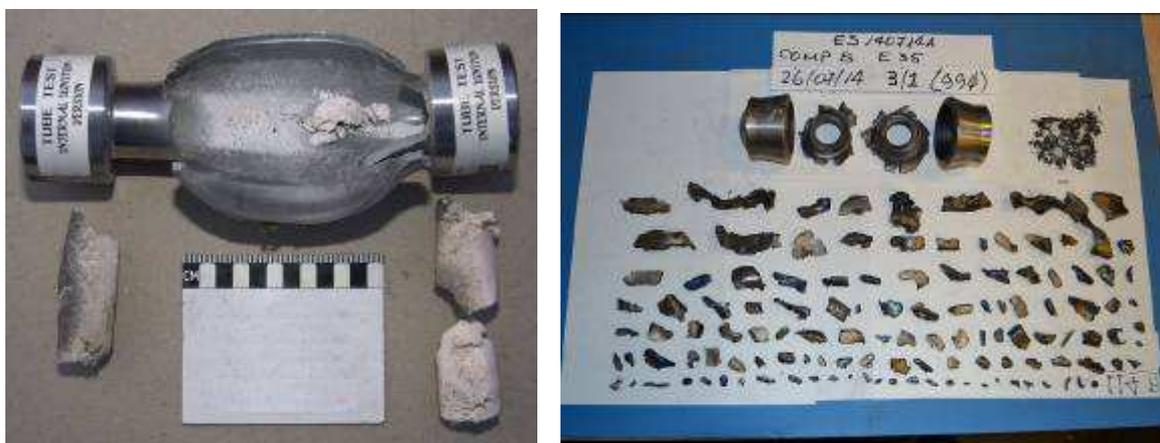
Figure 3. Internal Ignition test good and poor responses for cast cured PBX and Comp B.
